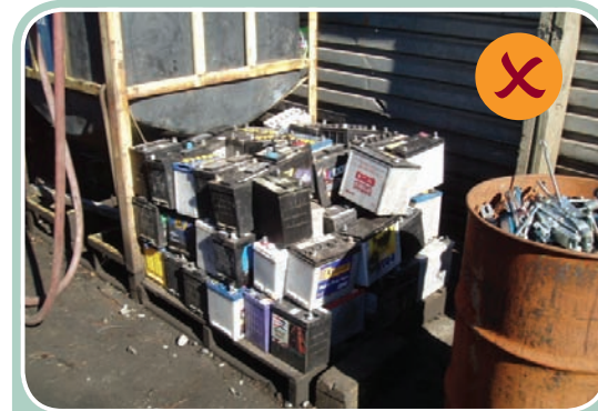
Batteries stored uncovered and on unsealed ground have the potential to leak into the stormwater system
