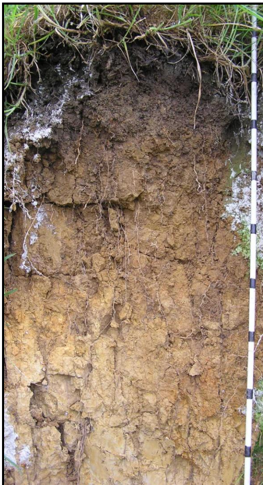
Figure 4. Low permeability Ultic Soils, showing coarse blocky structures and grey mottling in the subsoil, on Waitemata Formation sandstone in the West Auckland area. (Scale in 10 cm increments. Note: the surface white material is hydroseeding mulch.)
